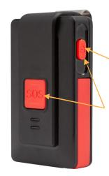
When off, press and hold for 3 seconds to turn the device on.
